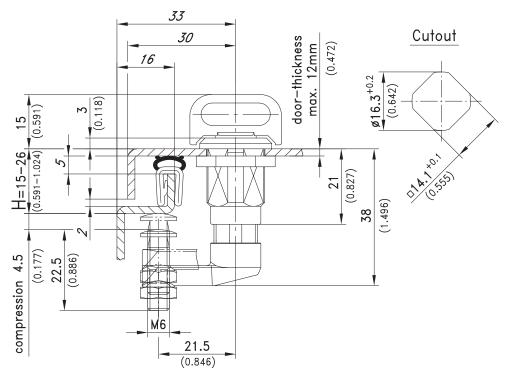
Position of cam and knob: "closed and compressed" "open"
